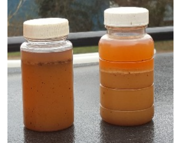
ALL THESE SAMPLES SHOW THAT BOTH TANK AND FUEL NEEDS CLEANING. FUEL SHOWING JUST HAZINESS IS SATURATED DIESEL. WATER MIXED IN WITH DIESEL AND WILL NEED CLEANING
