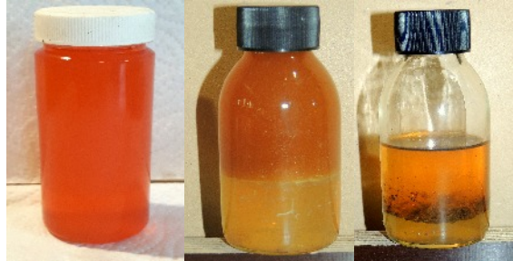
SATURATED DIESEL WATER & DIESEL
