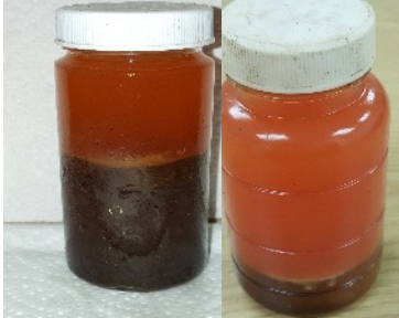
RUST WATER WITH DIESEL BUG SITTING ON WATER SURFACE
